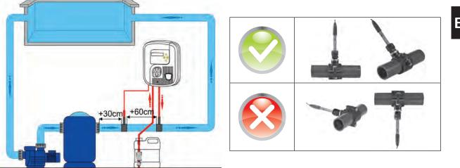
• The liquid chlorine injection point must be positioned before a pH corrector injection point and after the heating system.
