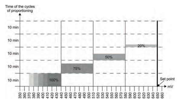
This proportional injection is cyclic and the cycle duration is 10 minutes. The dose will change according to the distribution of injection times and pauses. The proportionality adjusts automatically and the balancing between the different doses is made in 70 mV steps.
